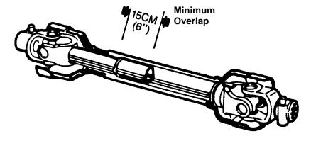
G. Clamp end of driveline in a vice. Cut off shield where marked. (Figure 2-3).
